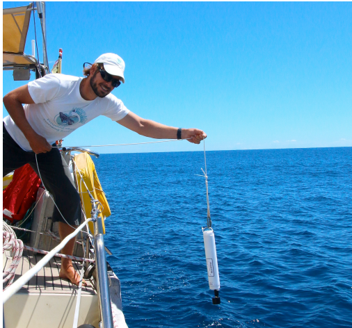
HHR New Zealand Expedition. Dr. Olaf Meynecke lowering a CTD to measure difference in temperature and salinity.
